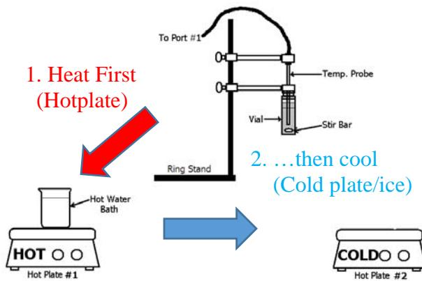
*entire ring stand apparatus* and reposition it over the cold stir plate. Continue stirring. Allow the vial to cool slowly. More dilute solutions may require the direct application of ice to reach cool enough temperatures in a *reasonable* amount of time.
