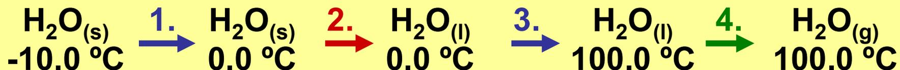
$$1. \quad q = m c_{\text{ice}} \Delta T = 500.\text{g} \times 2.10 \text{ J/g}^\circ\text{C} \times (0 - -10.0^\circ\text{C}) = 10500 \text{ J}$$
