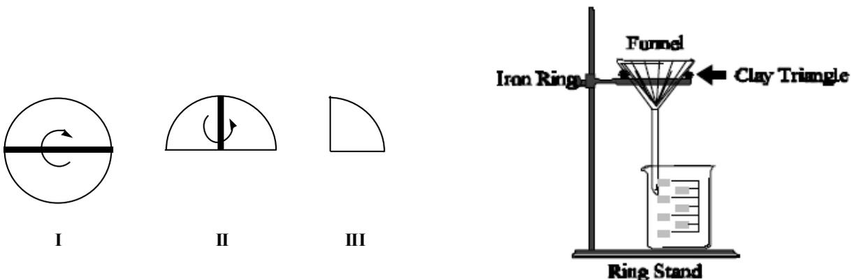
3. Set up a funnel with filter paper (see the diagram above on the right). The funnel should be supported on a ring stand. The folded filter paper is placed in the funnel and wetted down with the solvent (distilled water) so that the paper adheres to the funnel. Place a 150 mL beaker under the funnel stem to collect the filtrate.
