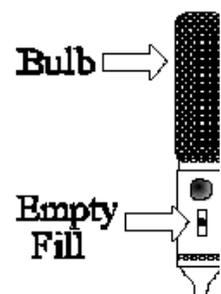
The droplet of liquid that remains stuck in the pipette after emptying should not be added to the dispensed liquid.
