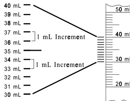
The examples below illustrate several volume measurements using graduated cylinders with different increments. Notice that the arrows indicate the position of the bottom of each meniscus.
